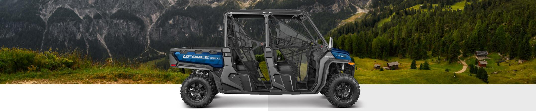
UFORCE 1000 XL provides switchable 2WD/4WD drive mode and 4WD drive lock function and is equipped with a CV-Tech transmission system.
